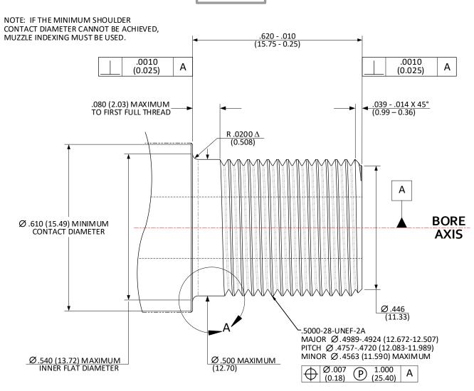
DATUM "A" FEATURE IS DEFINED AS THE LAST 3.0000 INCHES (76.200) OF THE BORE AT THE MUZZLE END OF THE BARREL.  $\Delta$  = REFERENCE DIMENSION (XX.XX) = MILLIMETERSDRAWING PREPARED USING THE DIMENSIONING CONVENTIONS DEFINED IN ASME Y14.5-2018.
