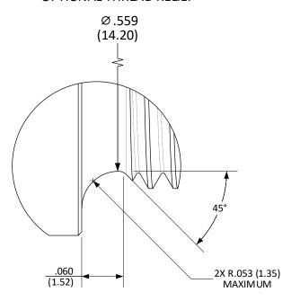
DO NOT SCALE FROM DRAWING UNLESS OTHERWISE SPECIFIED DIMENSIONS ARE IN INCHES
