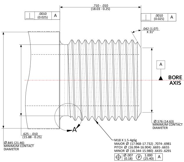
NOTE: IF THE MINIMUM SHOULDER CONTACT DIAMETER CANNOT BE ACHIEVED, MUZZLE INDEXING MUST BE USED.
