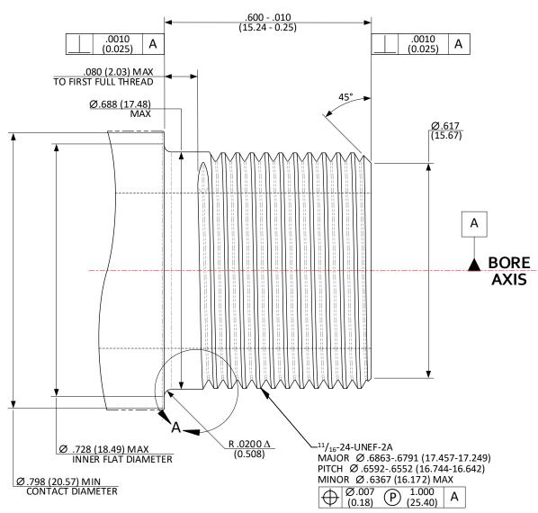
NOTE: IF THE MINIMUM SHOULDER CONTACT DIAMETER CANNOT BE ACHIEVED, MUZZLE INDEXING MUST BE USED.
